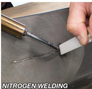
Repair instead of replace. Insurance companies want plastic parts repaired to keep replacement costs down, preventing possible loss. Welds most plastic parts used in today's vehicles'.
